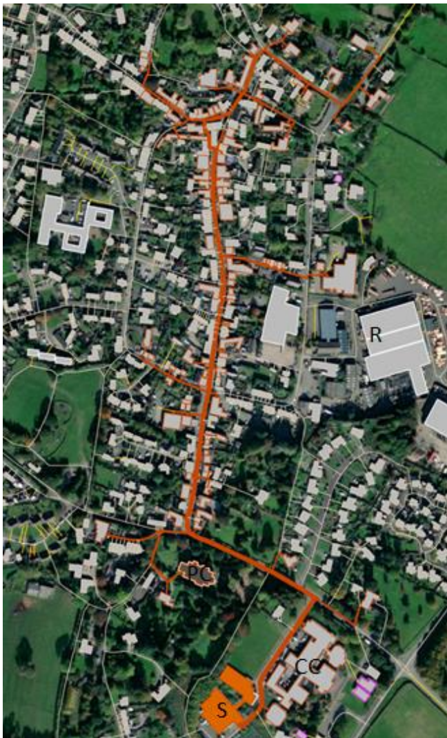
Figure 12 Proposed larger heat network based on heat pumps
